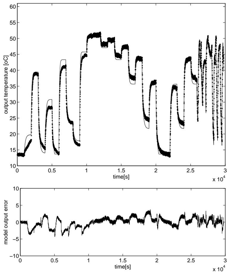
Figure 5: The validation of the Nonlinear Generalized Output Error model.
