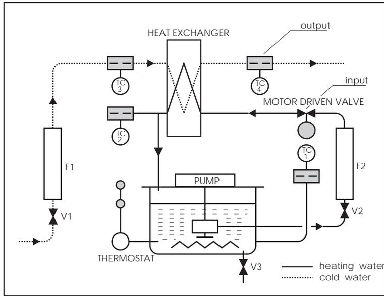
Figure 3: The scheme of the laboratory scale heat exchanger.
