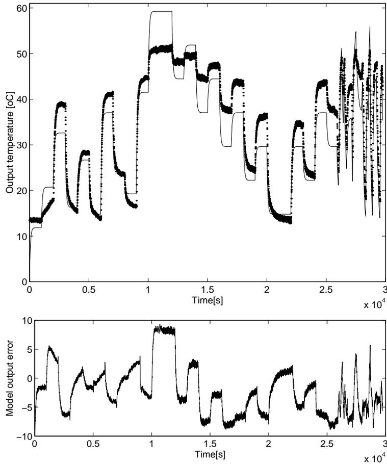
Figure 4: Comparison of the responses of the linear nominal model and the measured plant.
