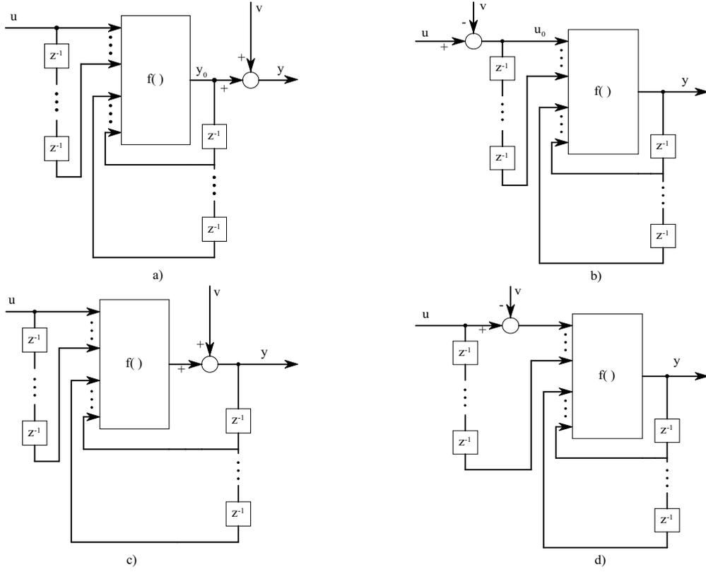
Figure 2: The representation of noise which results in an unbiased estimation for the output error (a), the input error (b), the generalized output error (c) and the generalized input error (d) models.
