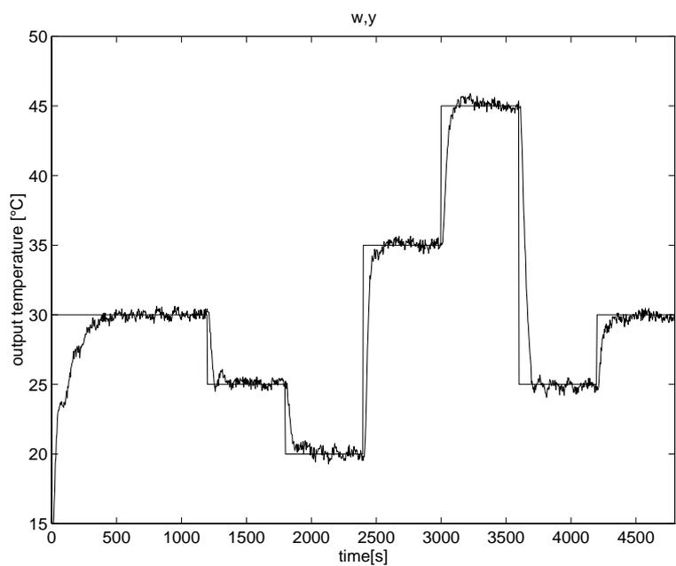
Figure 6: The closed loop response of the Nonlinear Output Error model based predictive control.
