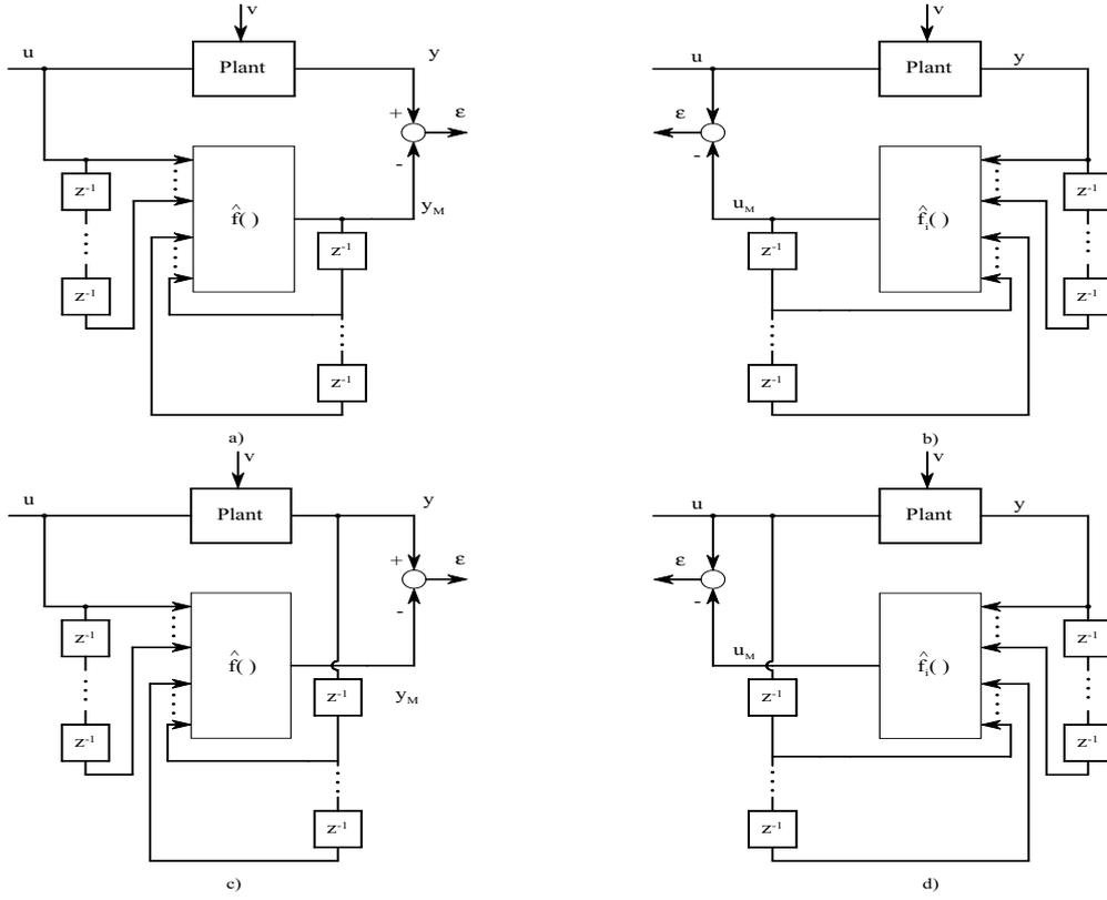
Figure 1: The output error (a), the input error (b), the generalized output error (c) and the generalized input error (d) identification models.
